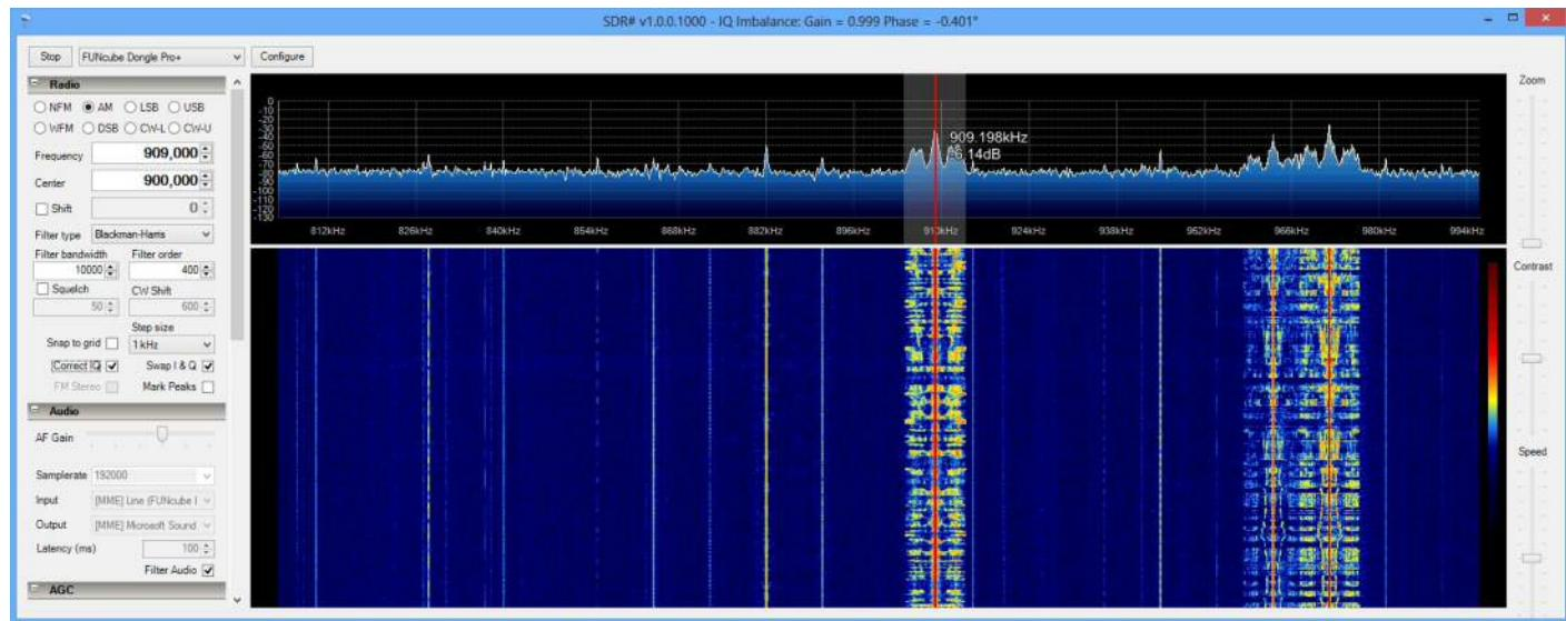
The reason to keep the center frequency a few kHz away from the frequency of interest when receiving narrowband signals like AM, SSB, NBFM and CW is that there are some artefacts from local oscillator phase noise that can interfere with signal reception.
