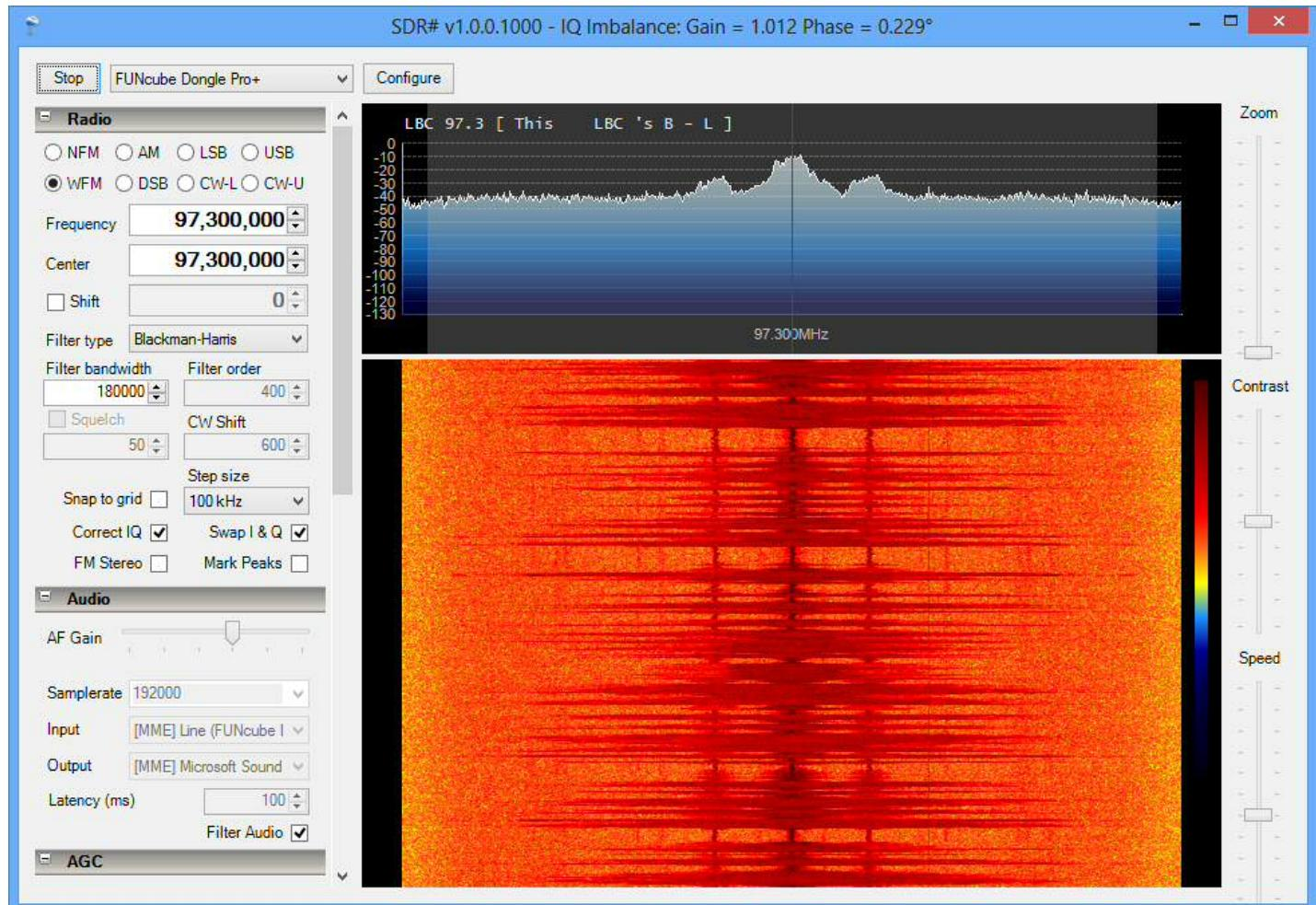
Broadcast FM is a fairly wideband signal. To receive narrowband signals such as on the AM broadcast band, set the Center frequency a few kHz away from the required frequency and then fine tune either by adjusting the Frequency setting or simply clicking on the spectrum display at the desired station. For example, below shows the reception of 909kHz on medium wave.
